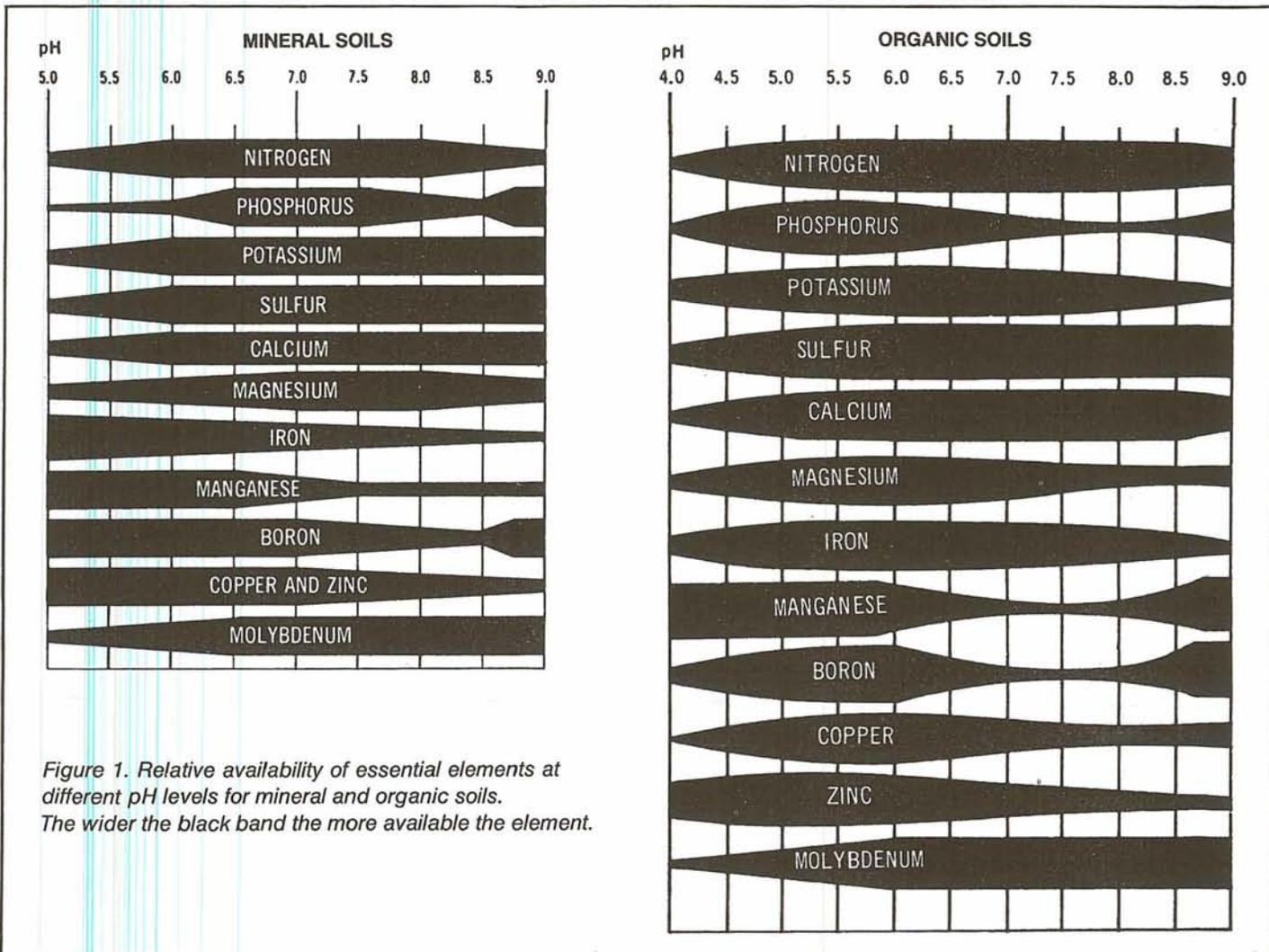
Figure 1. Relative availability of essential elements at different pH levels for mineral and organic soils. The wider the black band the more available the element.
